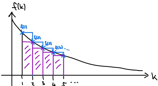
$$\left. \begin{aligned} \text{blue area} &= \sum_{k=1}^N f(k) \geq \int_1^N f(x) dx \\ \text{purple area} &= \sum_{k=2}^N f(k) \leq \int_1^N f(x) dx \end{aligned} \right\} \Rightarrow \sum_{k=2}^N f(k) \leq \int_1^N f(x) dx \leq \sum_{k=1}^N f(k)$$
