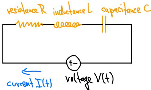
The voltage between two points is the same:  $V(t) = V_R + V_L + V_C$
